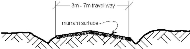
Side Drain Ditch - depth of ditch will vary along the length of the run between turnout or outlet
