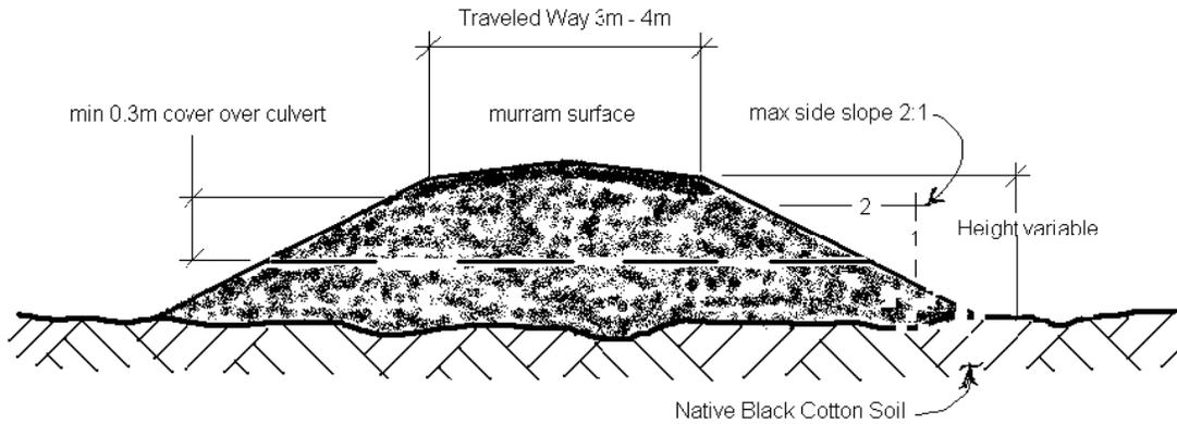
Note: Reapply surface vegetation and surface soil to new fill slopes to aid in revegetation
