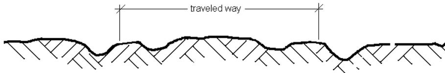
Typical road cross section after filling up the longitudinal ruts by reshaping the road
