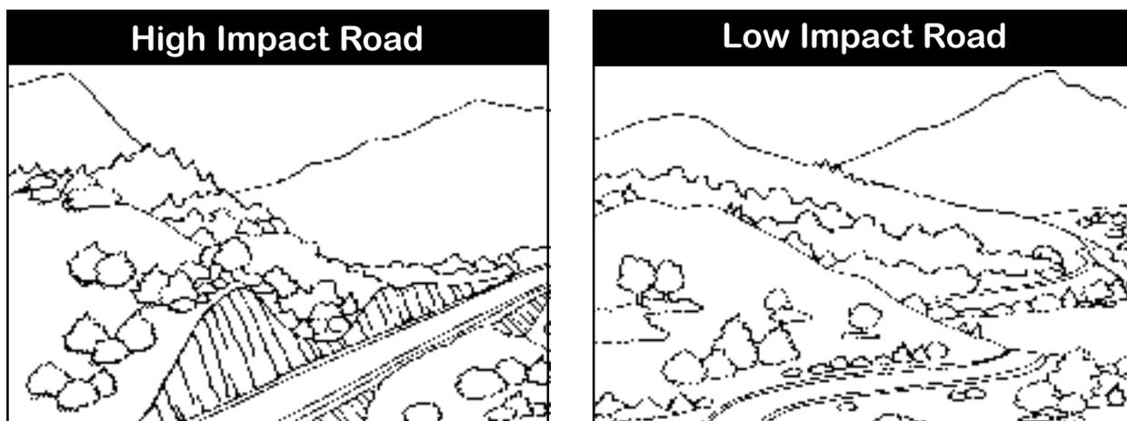
**Figure 2.1** Low versus High Impact Roads: These figures show the reduced work and reduced environmental impacts from low standard roads that conform to the topography. The low standard road reduces cut and fill slope size, reduces earth work, visual impacts, and minimizes changes to natural drainage patterns. The high standard road can move a large volume of traffic rapidly and safely.
