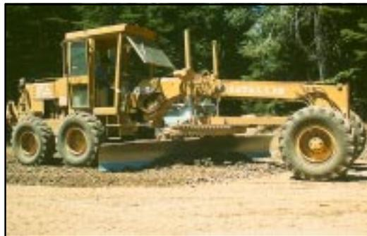
**Photo 4.10** Use grader maintenance to keep the road surface properly shaped and drained.
