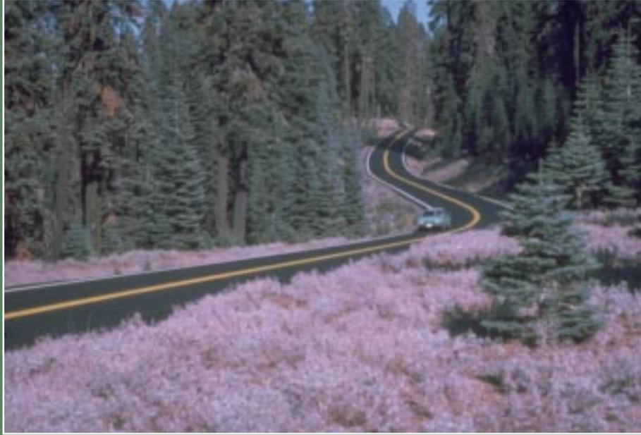
*The paved road (above) and gravel road (below) are relatively well located and designed low-impact roads since their surfaces are armored and they conform to the terrain, thus dispersing water effectively and avoiding heavy earthwork.*
