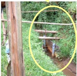
Topsoil loss from slopes upstream in the watershed (top) is assessed with a visual turbidity monitor (bottom).
